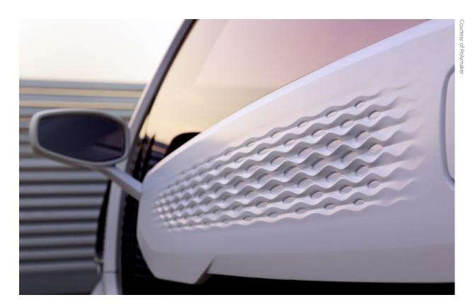
The ambitious project of Italian car manufacturer XEV and 3D-printing company POLYMAKER resulted in LSEV, the first 3D-printed electric automobile. The lightweight high-grade plastic used to make the vehicle encouraged the engineers to reduce the number of printed components from over 2,000 to 57. This combination of mass-scale manufacturing and easily accessible design can be adapted to the operations of countless other industries.
